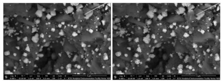
Surface morphology of the QD media (SEM imagery): initial state (left); metallic state 55 seconds after exposition to the SEM electron beam (right)
